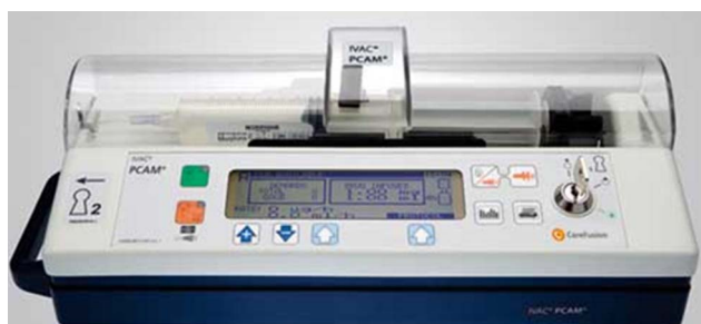
Figure 1 Syringe pump (IVAC PCAM) 21 currently used in Evelina London Children's Hospital.
