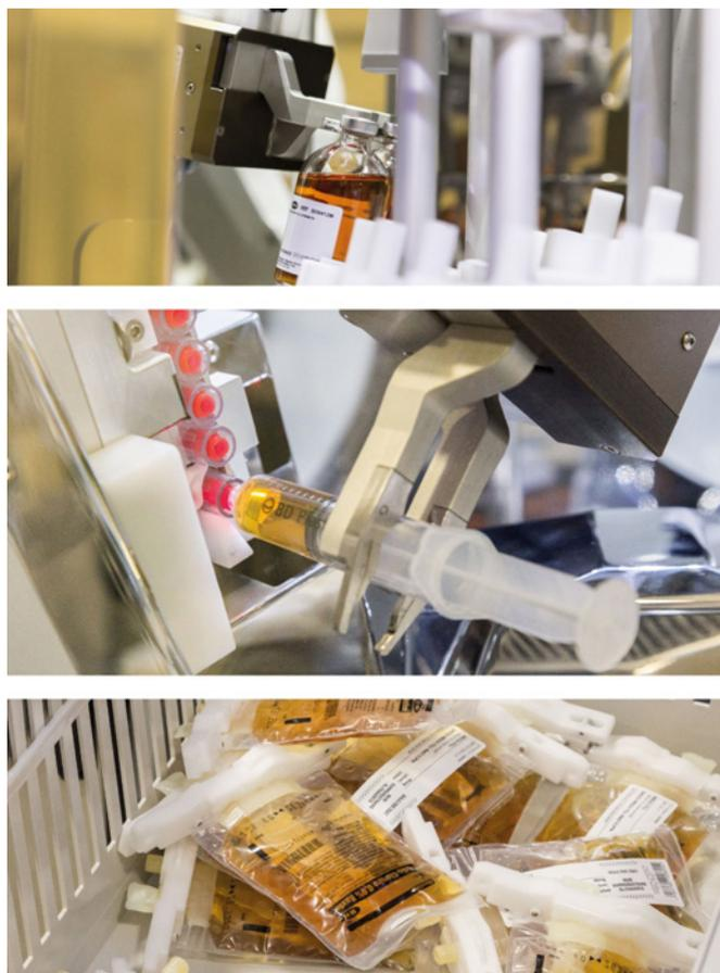
**Figure 4** Media Fill test. Respectively phial, syringe and bag manipulation.
