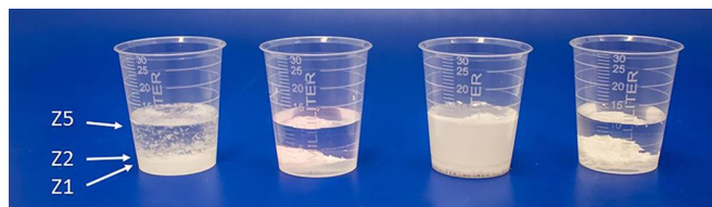
Figure 1 The four aspirin tablets upon passive dispersion in 10 mL purified water for 3 minutes. From left to right: Dispersible Aspirin (75 mg), Bayer Chewable (81 mg), Disprin (300 mg), Aspirin (500 mg). Zones 1, 2 and 5 are marked Z 1, Z 2 and Z 5, respectively.
